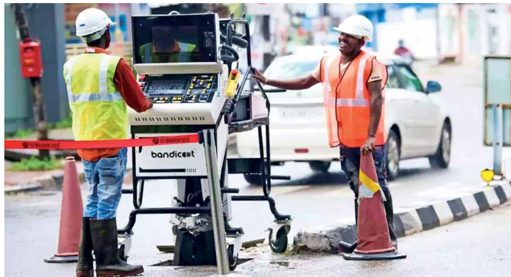
Bandicoot, a robotic machine, cleans sewer manholes
